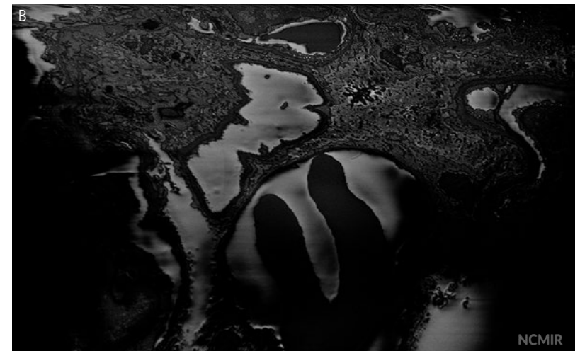
Block face images of mouse lung tissue (A) with Focal Charge Compensation and (B) without Focal Charge Compensation. Scale bar: 1 micron. Images: courtesy of NCMIR, University of San Diego, US.
