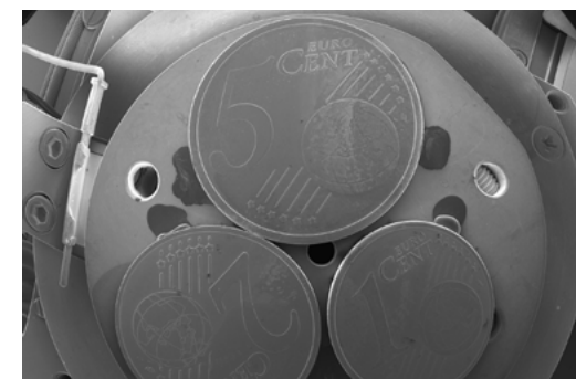
Overview mode offers an extremely large field of view and enables an easy navigation and fast relocation of ROIs. Image is taken at 5 kV using the SE2 detector.
